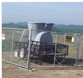
SODAR unit in operation at ICG's Cowan surface mine complex
